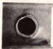
Illustrating completely smooth finish of swaging of rung to stile.
